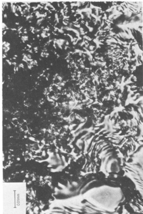
Figure 1 Photomicrograph of MgO after interaction with Re at 2450° C for 20 min.
